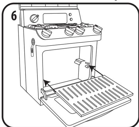
6 To insert the shelf, slide the sides of the shelf in between the brackets in the oven.
